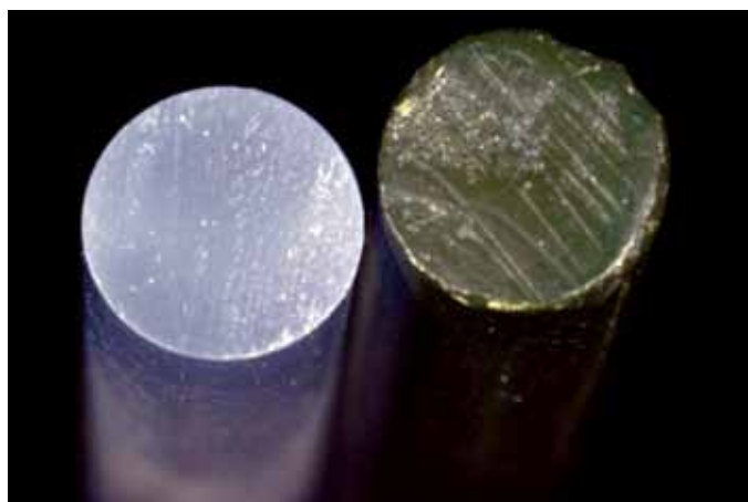
1 Hot glue stick (7 mm in diameter) and green stick compound with similar diameter.
