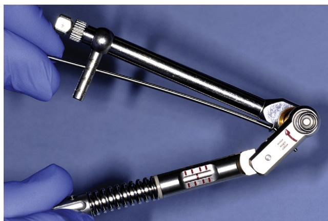
**Figure 7.** Two mechanical torque limiting devices coupled (Note: beam wrench reading in error, requires calibration or replacement.)
