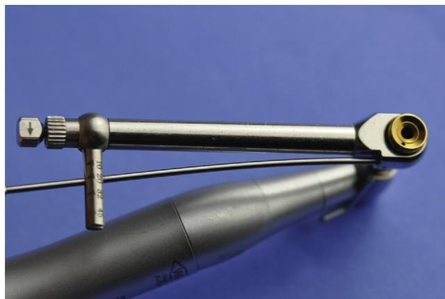
**Figure 6.** Coupling electric torque delivery to mechanical beam torque wrench.
